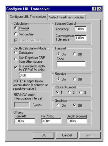
See the LBL ACOUSTICS chapter of the WinFrog User's Guide for details on setting these parameters. They are the same across all LBL TRANCEIVERS except for the **Transmit Code**. The "transmit code" to enter for a DS7000 is the Receive frequency of the fixed transponders.
